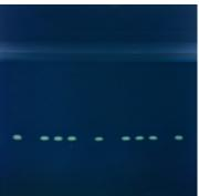
**Figure 4.** TLC Analysis of plate by the TLC Explorer under VIS excitation (top) and UV 366 nm excitation (bottom). The tracks 1, 5 and 9 are the references of dexamethasone and 2-4 and 6-8 are the samples. The plates were derivatized with a mixture of dihydroxybenzaldehyde, glacial acetic acid and sulfuric acid.
