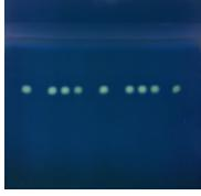
**Figure 5.** TLC Analysis of plate by the TLC Explorer under VIS excitation (top) and UV 366 nm excitation (bottom). The tracks 1, 5 and 9 are the references of dexamethasone acetate and 2-4 and 6-8 are the samples. The plates were derivatized with a mixture of dihydroxybenzaldehyde, glacial acetic acid and sulfuric acid.
